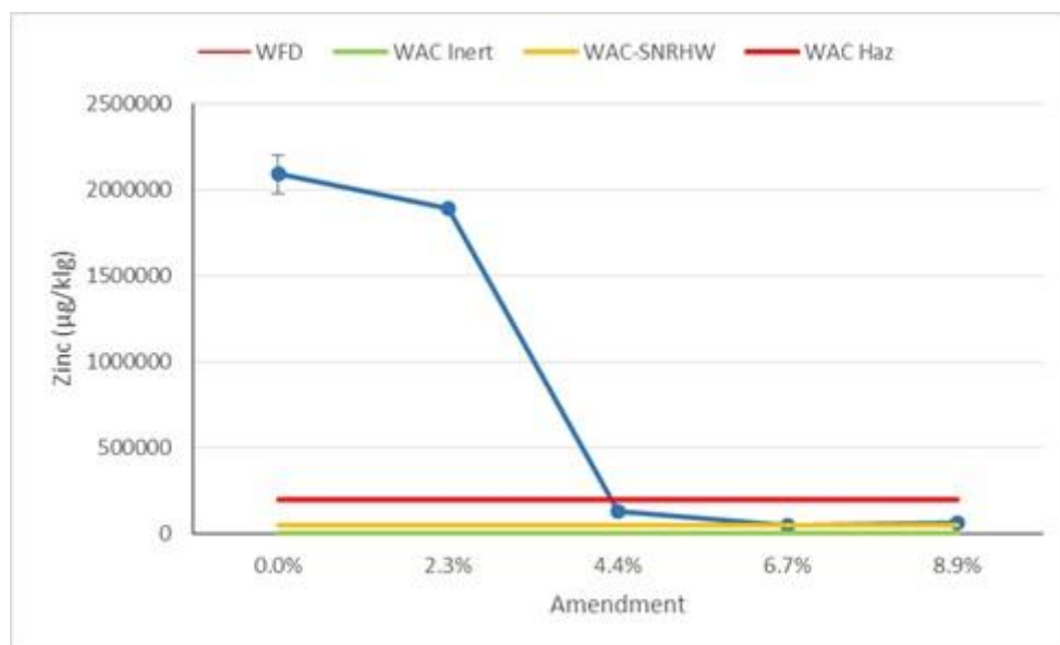
Figure 39. Concentrations of leachable zinc (µg/kg) in soil taken from site S3 before and after treatment with either 2.3, 4.4, 6.7 or 8.9% (w/w) C-Cure metal adsorbing product (TTLX). N=2. Thin red line represents annual average EQS for EU surface waters; light green line is the Waste Acceptance concentration for inert waste and
